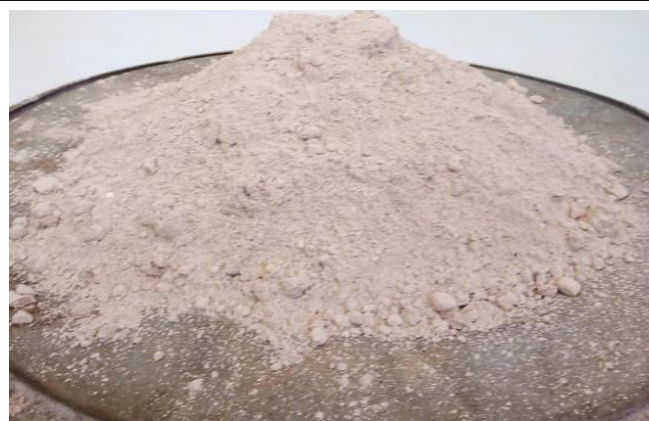
Figure:5 Views from waste ceramic powder from disposedsite.
